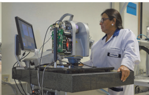
Figure 11: Final assembly and balancing
