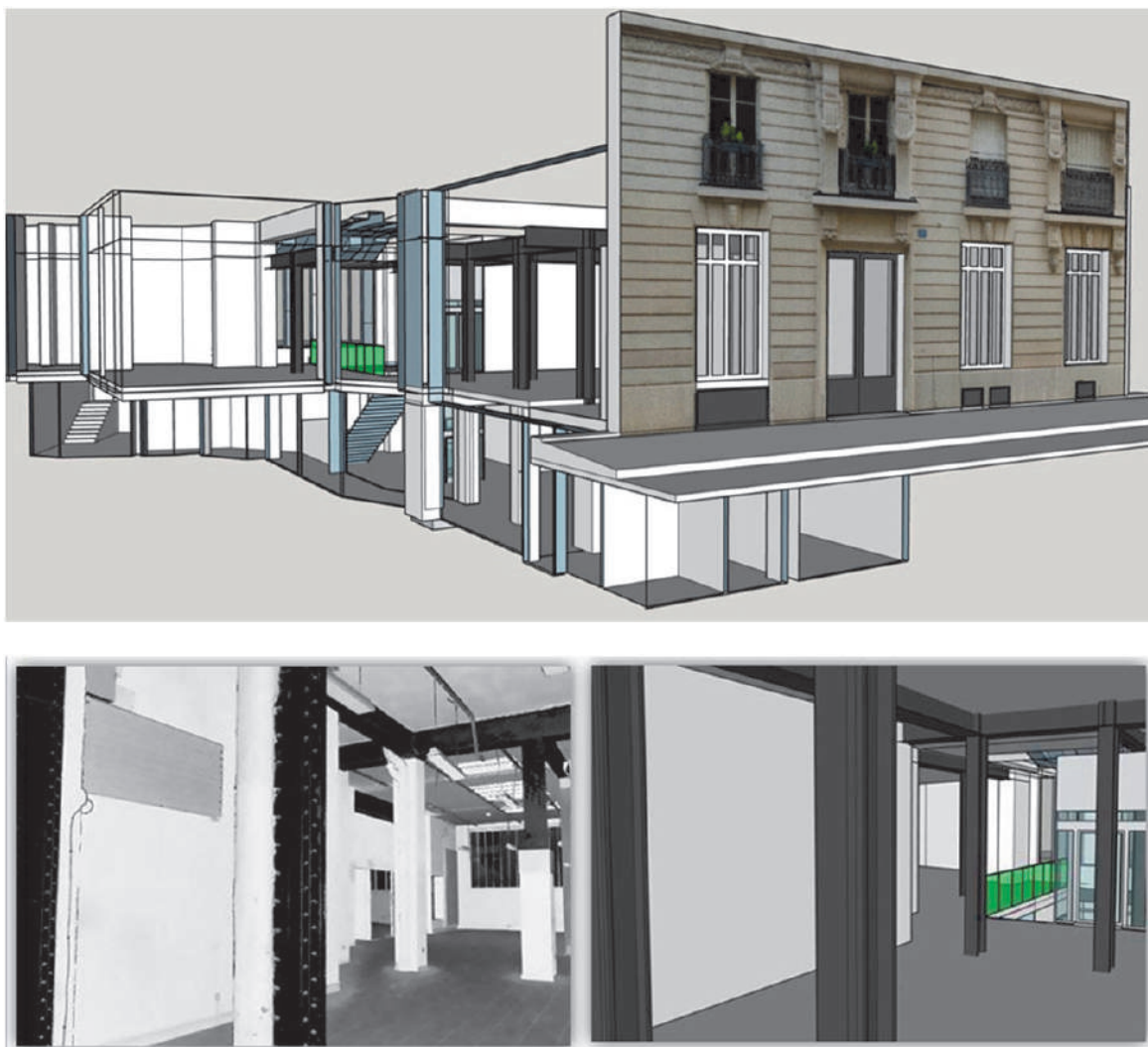
Figure 7: Trimble TX8 scans modeled in SketchUp for a building renovation project.
