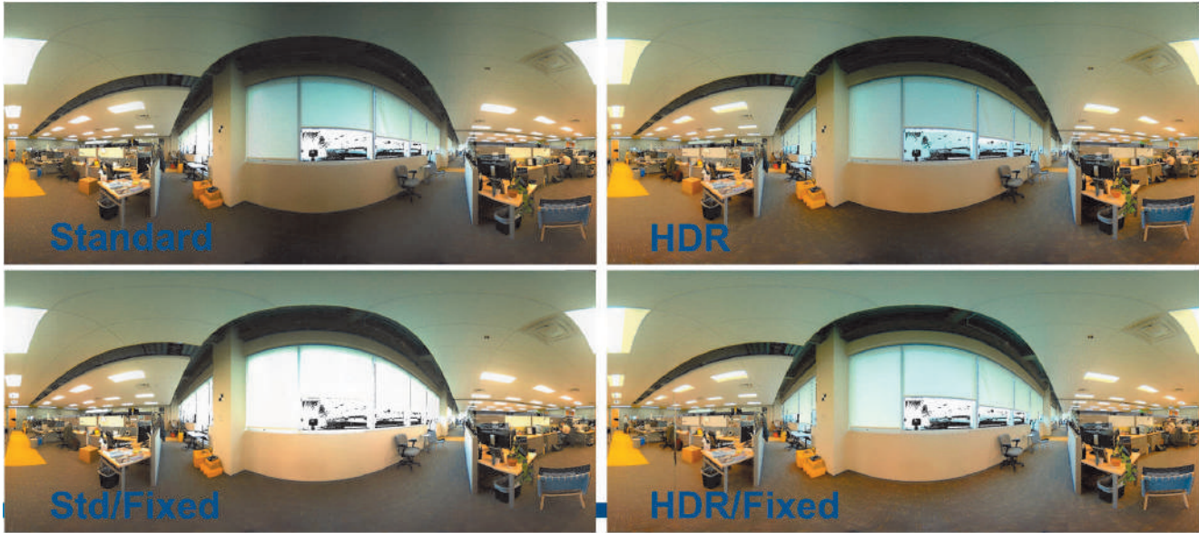
Figure 3: Comparison of Auto and Fixed exposure for Standard and HDR modes
